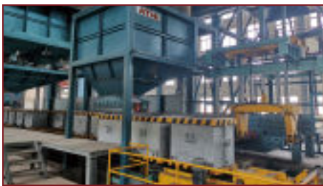
Shell casting line
