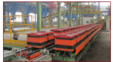
Lost foam casting production line
