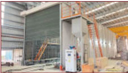
QAT2610 Sand Blasting Room
